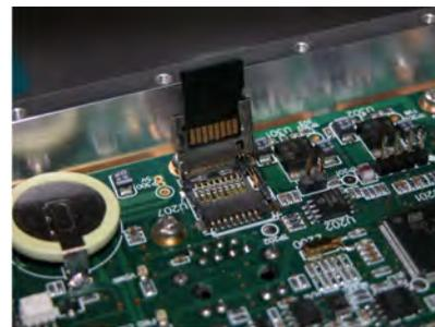
10. Close the holder by pressing the cover down and sliding it towards the edge of the PCB (in the direction of the LOCK arrow on the holder) until it clicks firmly into place
