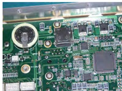
8. Open the microSD card holder by using your fingernail to slide the holder towards the centre of the PCB (in the direction of the OPEN arrow on the holder). The holder will then pop up slightly
