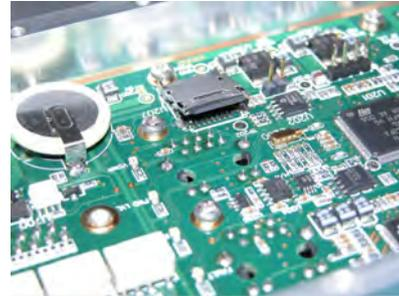
9. Swap the microSD cards by opening the holder fully, noting the orientation of the card
