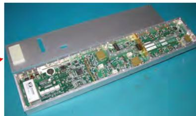
7. Find the microSD card holder on the PCB between the microprocessor IC and the battery
